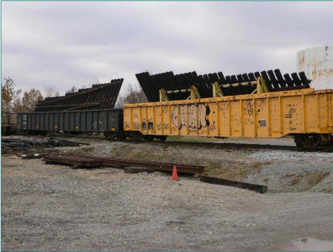
Left: Bill Heaton took this photo of CSX Snap Track loaded in gons, ready for action at Atkinson Yard, Madisonville, KY.. This would be a simple, but effective modeling project in any scale.
